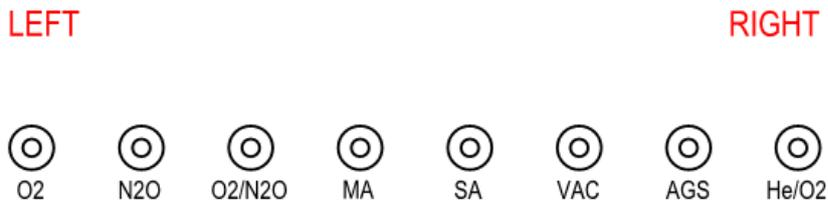
**Figure 2: Wall mounted terminal unit mounting order – vertical array**
